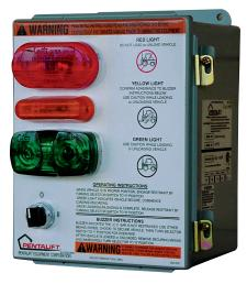
NEMA 12 interior wall mount control station. High visibility interior signal lights are coordinated with exterior signal lights. Clear, concise and easy to follow instructions guide dock attendant on how to use the system. Selector switch and amber light accommodate "override" mode. CSA certified for the design and manufacturer of industrial control equipment.
