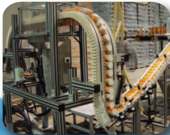
Gripper Conveyor System
